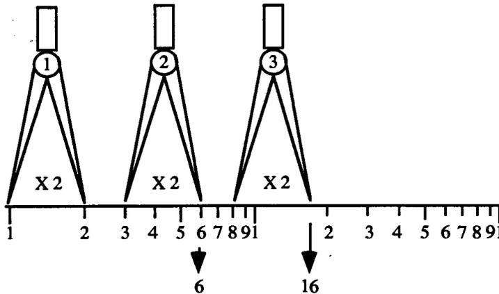
For example, to multiply 2 times 3, we place the left point of the x2 divider on 3, and read the product 6 opposite the right divider point. See divider 2 above. To multiply 2 times 8, we place the left point of the x2 divider on 8, and estimate the product 16 on the line opposite its right divider point. See divider 3 above. To divide you subtract the distances with the divider.
