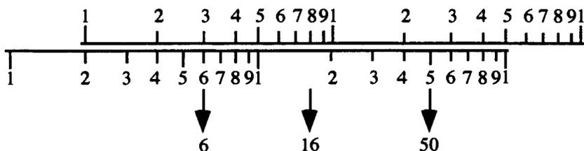
To multiply using Oughtred's slide rule, we set the left index of the top line to the multiplier "times 2". Now the product of 2 times every number in the top line is directly below it in the bottom line. Directly below 3, we find 6. Directly below 8, we interpolate 16. Directly below interpolated 25, we find 50.
