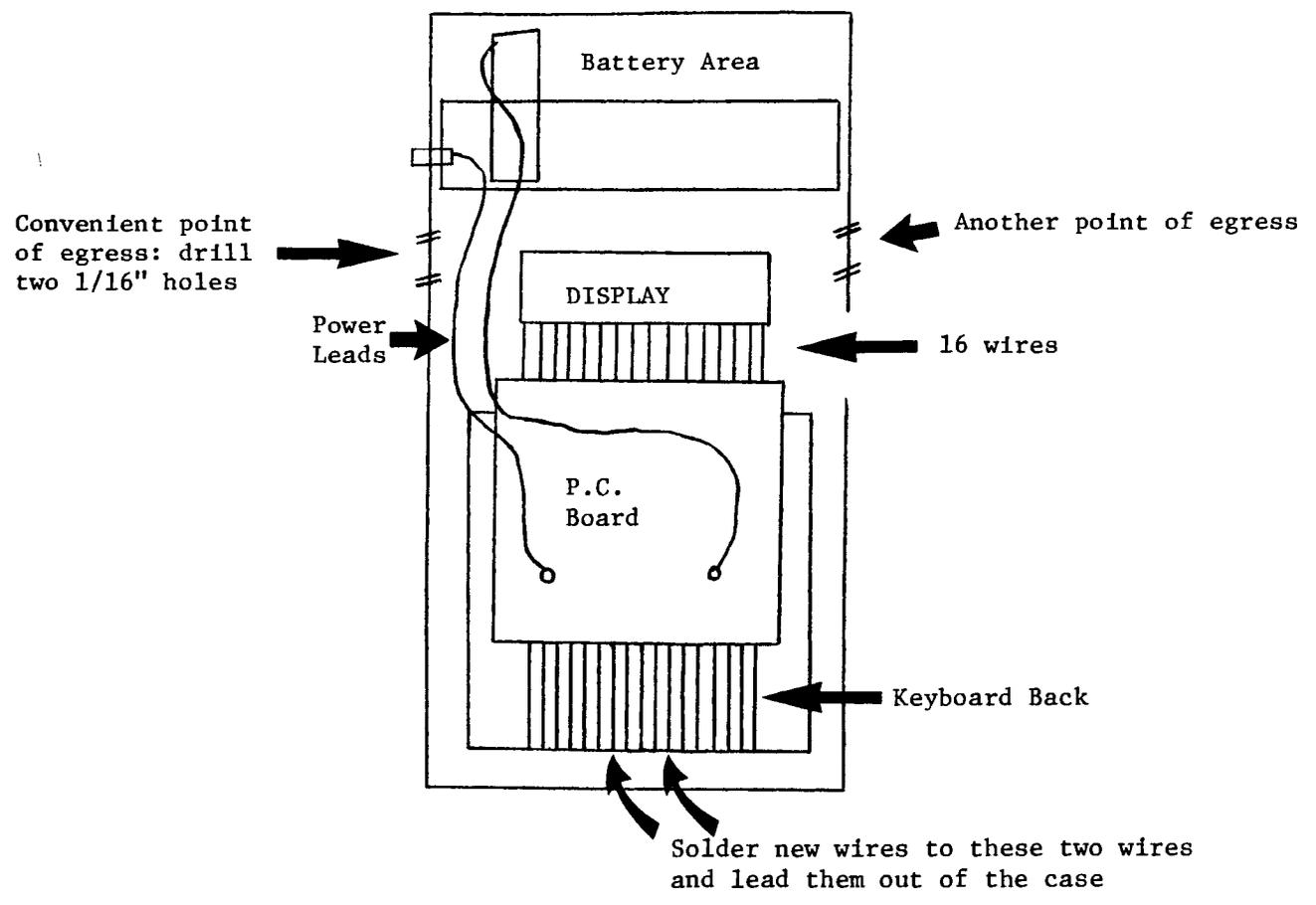
Diagram 1. Converting a Unisonic 1541L Calculator to a Counter with a Wide Variety of Applications
